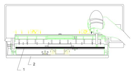
1. Calibration Board 2. Scanner Front Door
