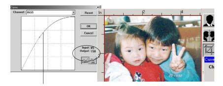
When the curve is moved up or down, the image turn brighter or darker.
